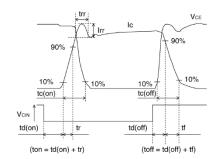
Fig.4 Switching time test waveform
