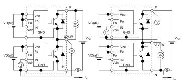
Fig.3 Switching time and SC test circuit
